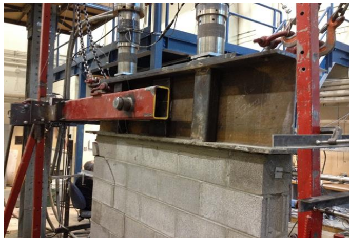
Fig 2: Load application mechanism.
